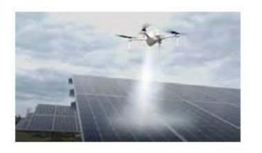
Conclusion: Through AI algorithm and software control, automatic UAV system can intelligently design flight path and assign tasks, break terrain restrictions and weather restrictions, automatically plan routes, automatically detect hot spots and accurately locate, and send information to the system platform in real time. It can be equipped with a cleaning system to wash PV modules block by block without dead corners, solve the problem of dust accumulation on the surface area of PV modules.
